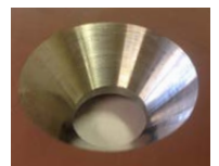
Counter Sunk-Hole in High-Tensile Wear Plate
