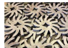
High Definition Plasma Cut 'Gears'
