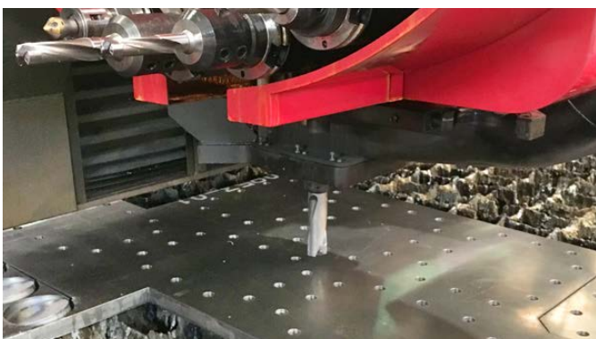
Drilled, Tapped & Counter-Bored Holes With Bevelled Edge
